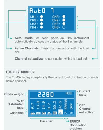
The TLM8 displays graphically the load cells response signal in mV for each active channel.
